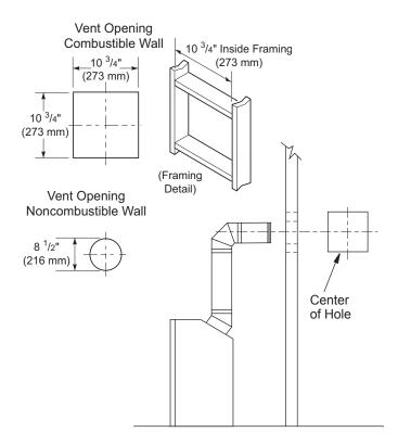
Figure 9 - Vent Opening Requirements
